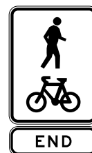
End shared path sign
